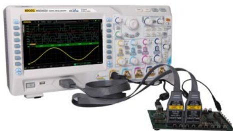
Figure 10 To Connect the Logic Probe
